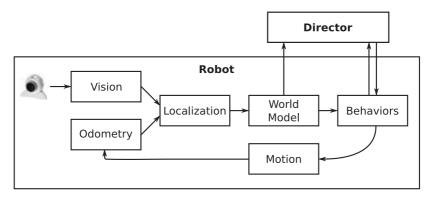
Fig. 3. The CMCast robot on-board behavior architecture.
