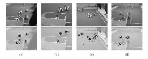
Fig. 5. A selection of interesting frames from the testing video. The top row shows the input frames. The bottom row shows the centroid voting space after running PCA-SIFT on the input frames. Each vote is annotated by a small black dot. The result of clustering and centroid-finding on this voting space is marked by larger black circles.
