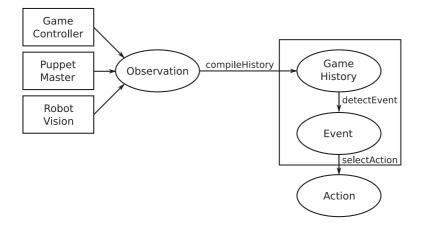
Fig. 8. The internal structure of the Director module of the CMCast global architecture (see Fig. 2).
